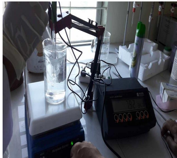
Figure 2: Using pH meter to get pH of 7.2 while making phosphate buffer
