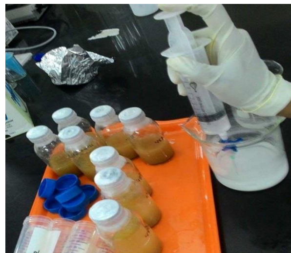
Figure 9: Using calibrated syringe to measure total gas and CH 4
