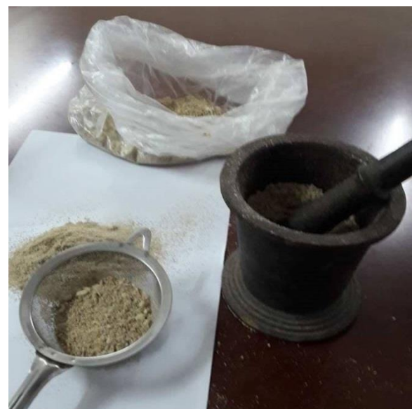
Figure 3: Commercial feed was powdered to <1mm size using mortar
