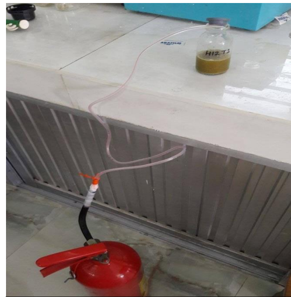
Figure 7: Using a small CO 2 cylinder to transfer 100% CO 2 to make the condition anaerobic
