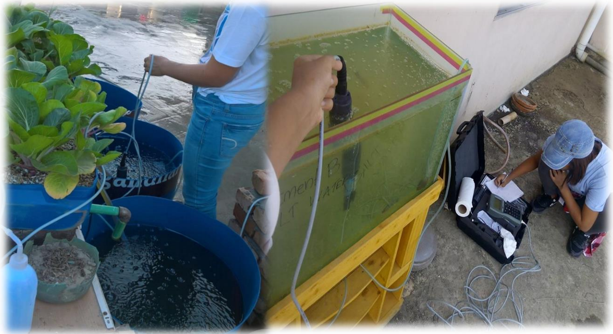
Figure 2: On-spot measurement of DO, TDS and pH using Hanna Instrument Multiparameter Meter
